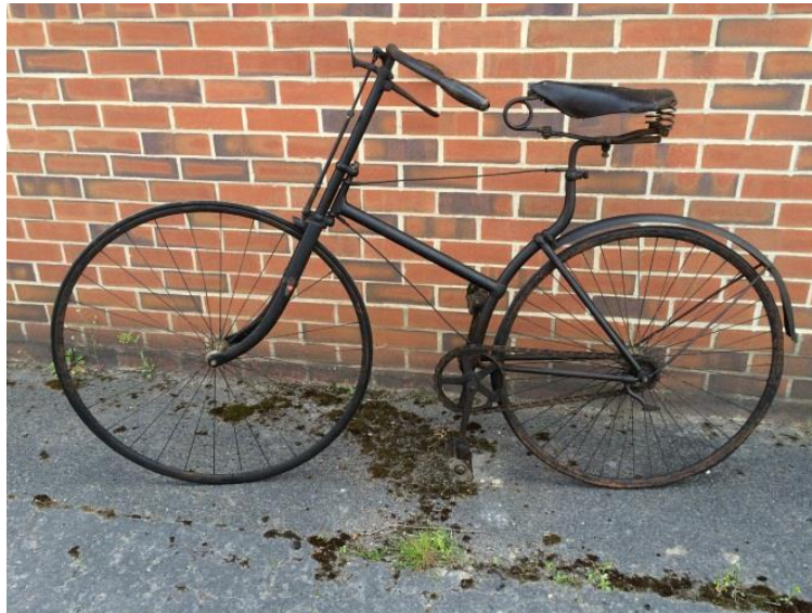
Our solid tyred safety bicycle c.1888 - the oldest bicycle going on display
